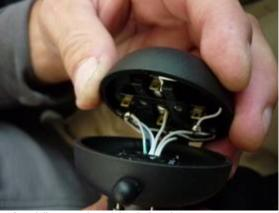
6. Carefully open the stick grip head. Inspect contacts and wires for quality of soldering, amount of solder on contacts (should be compact solders, large blobs are not acceptable). Inspect the insulation of wires for obvious wear. In case of damage, repair in accordance with FAA AC 43.13.
