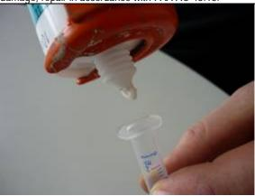
8. Fill up a small amount (10 ml) of silicone adhesive into a syringe if not using a smaller 82ml tube.
