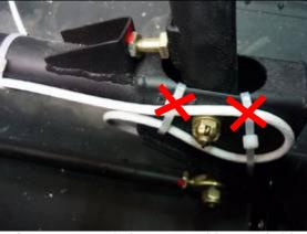
4. Cut two tye wraps in the root area of the control stick.
