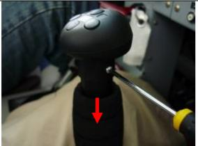
3. Pull down the foam stick grip and remove two locking screws on sides of the control stick.
