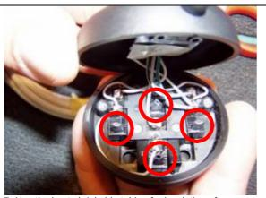
7. Use the heat shrinkable tubing for insulation of any unused contacts.
