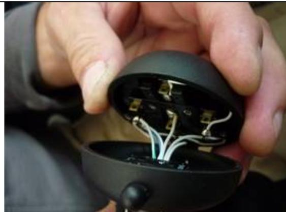
6. Carefully open the stick grip head. Inspect contacts and wires for quality of soldering, amount of solder on contacts (should be compact solders, large blobs are not acceptable). Inspect the insulation of wires for obvious wear. In case of damage, repair in accordance with FAA AC 43.13.
