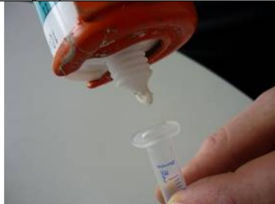
8. Fill up a small amount (10 ml) of silicone adhesive into a syringe if not using a smaller 82ml tube.
