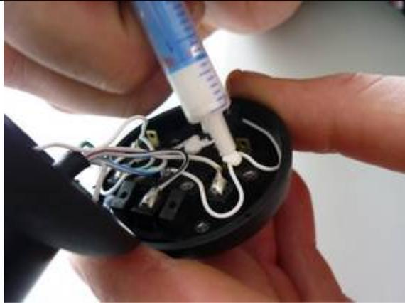
9. Dab a small drop of silicone adhesive on each of the contacts. Do not forget the PTT switch contacts (on lower part of the stick grip head) and fix heat shrinkable tubing on any unused contacts. Let it cure in accordance with the silicone adhesive manufacturer's technical data.
