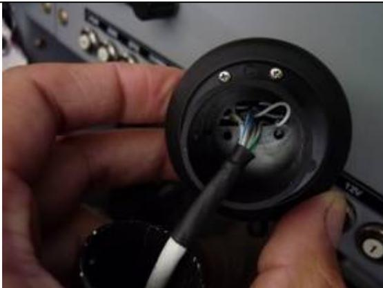
5. Lift the stick grip head up and remove four screws on its bottom side.
